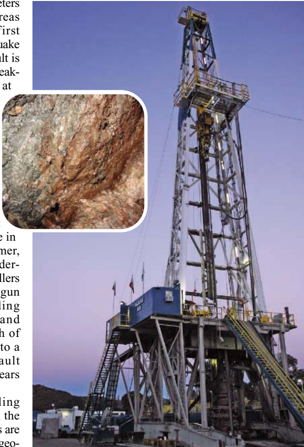
Deep reach. Scientific drilling into the San Andreas found a weak fault and retrieved altered and deformed fault rock (inset).
